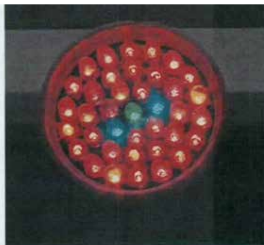
LED Grow Light, showing color caps on the individual LED lamps
